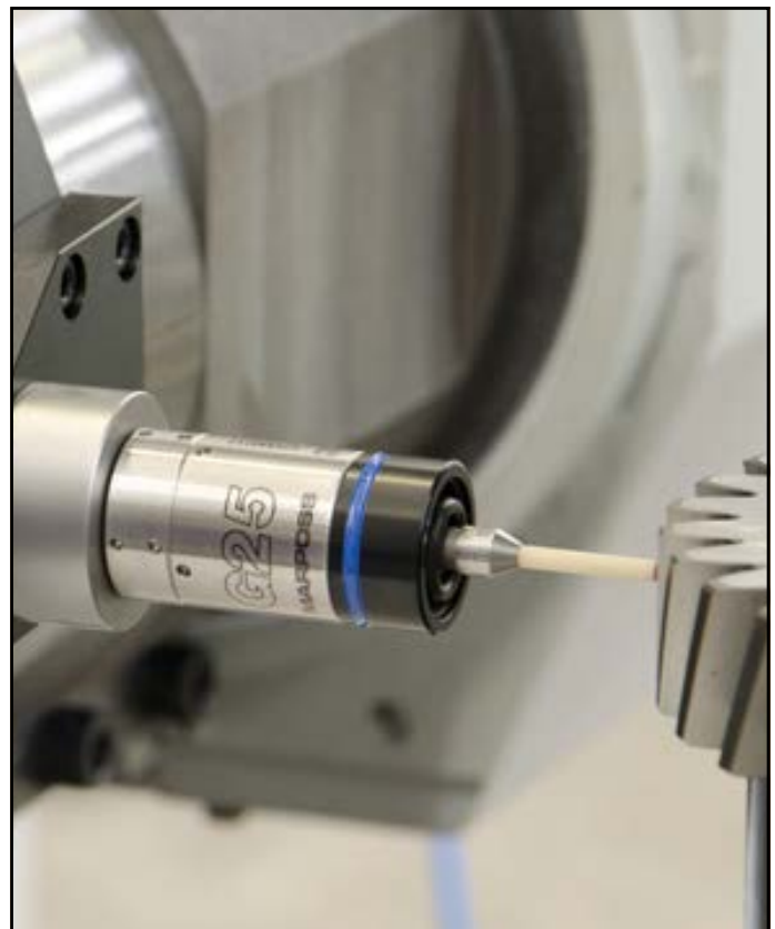
Figure 13 Scanning probe installed on a form gear grinding machine.
