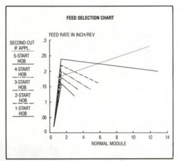
Fig. 5-Roughing cut feed rate chart.
