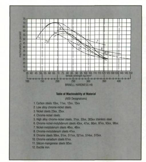
Fig. 2-Machinability in reference to workpiece material.
