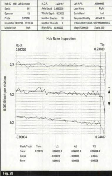
the rake line crosses the hob center. The rake offset is negative if the rake line makes an obtuse angle with the tooth outside diameter, and positive if the rake line causes an acute angle with the hob outside diameter. Most hobs have  $0^{\circ}$  rake, although there are some hobs with positive or negative rake. Rake is measured on the tooth face as shown in Fig. 25. The task of inspection is to find out rake deviation from the design geometry.
