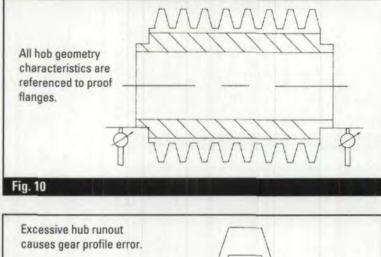
causes gear profile error. Gear profile error Gear profile error = Eccentricity \* 2 \* Sin(Axial Pressure Angle) Fig. 11 the hobbing process.
