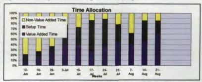
Figure 11-Time allocation breakdown during carbide hobbing trial.
