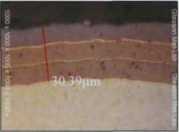
Figure 7—Coating fractures can contribute to poor hob performance. Multiple coating layers chipped on the outer surface (top), while the lower coating layers have remained intact (bottom).
