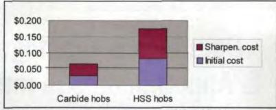
Figure 9-Cost-per-gear comparison between carbide and HSS hobs.
