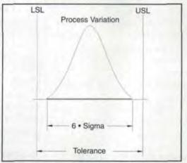
Figure 13-Improving process variables resulted in process variation becoming smaller than the tolerance.
