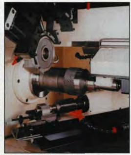
Figure 3-New CNC hobbing machine.
